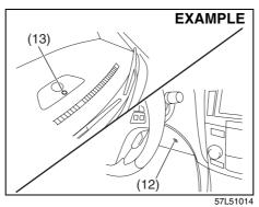
Be careful not to cover the interior temperature sensor (12) located between the steering wheel and the climate control panel, or the solar sensor (13) located at the top of the central part of the dashboard. These sensors are used by the automatic system to regulate temperature.
